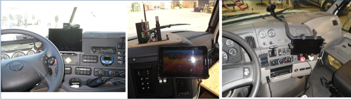
Figure 30. Placement of the Display Screen in the Integrated Truck (left), RSD1 (middle), and RSD2 (right)
