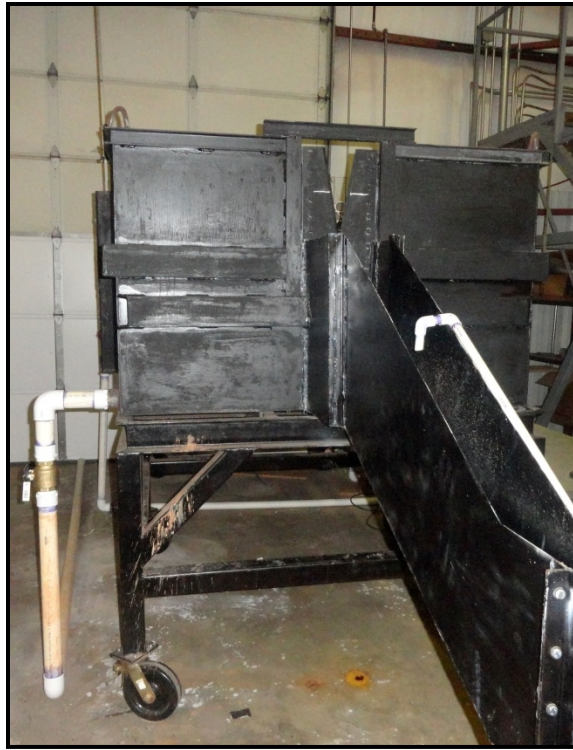
Figure 6. Constant head tank as constructed.
