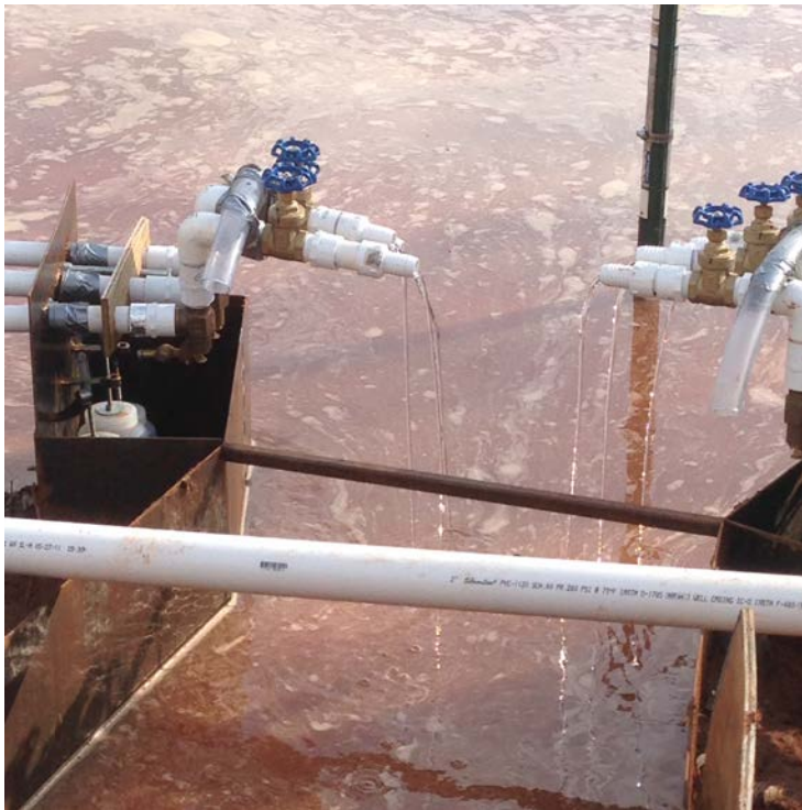
Figure 178. Updated valve and float system
