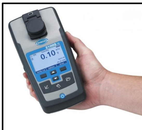
Figure 162. The 2100Q Hach turbidity meter used to test the turbidity for the jar tests.
