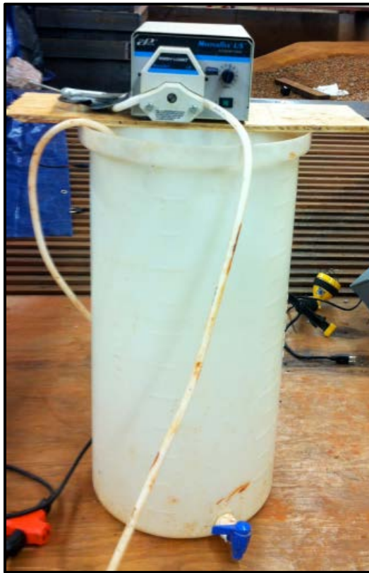
Figure 7. Flume flocculant injection system.
