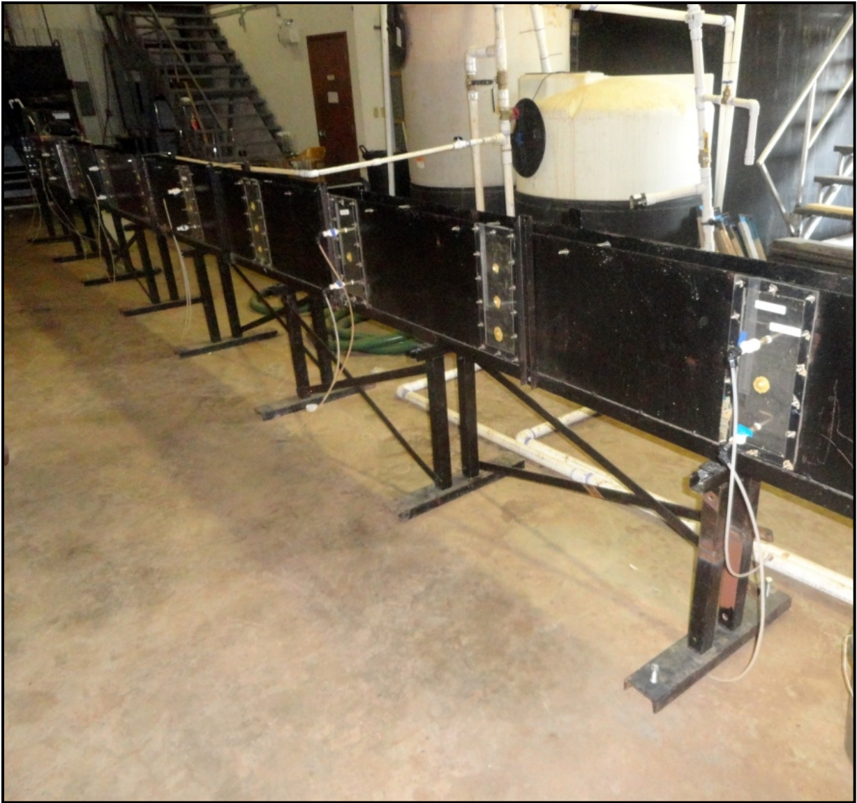
Figure 9. Flume apparatus used for determination of flocculation constants.
