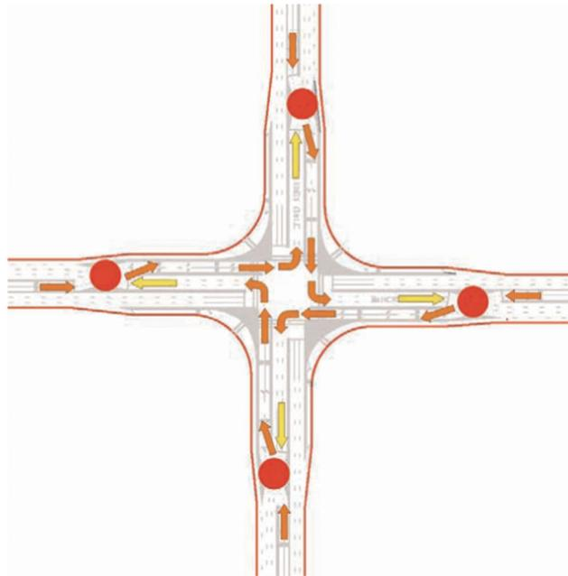
Figure 13.3 Full displaced left-turn intersection (9).
