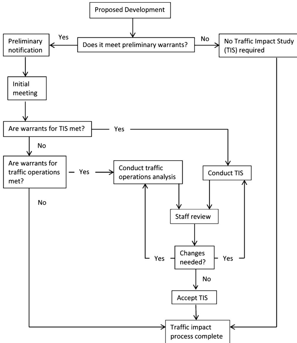
Figure 3.1 Flowchart showing the traffic impact study procedure.
