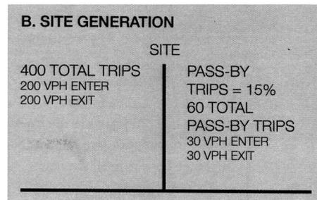
Figure 11.3 Application of pass-by trips.
