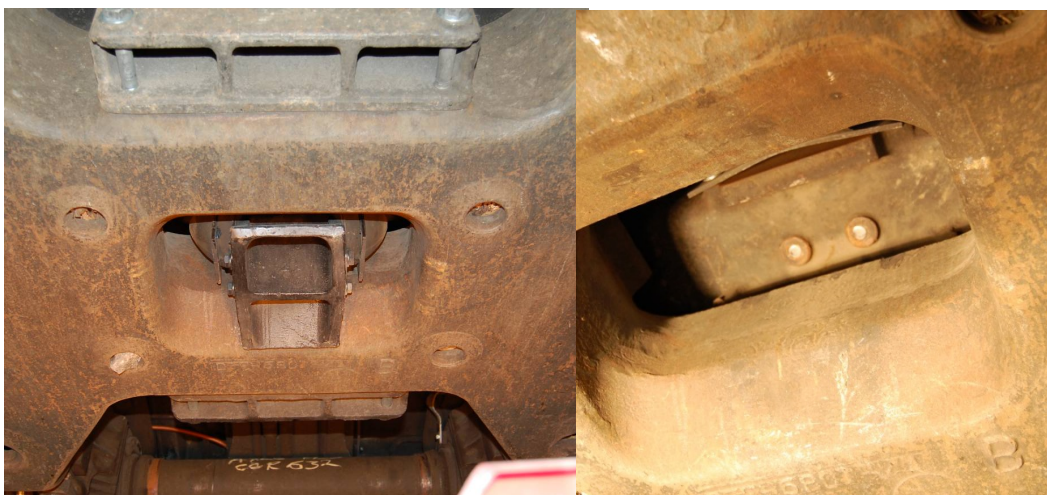
Figure A.2.1-15. Intact Truck Retention Mechanism
