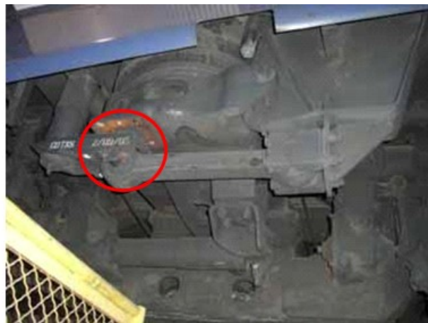
Figure A.2.1-12. Second Passenger Car Sidewall and Truck Attachment Damage
