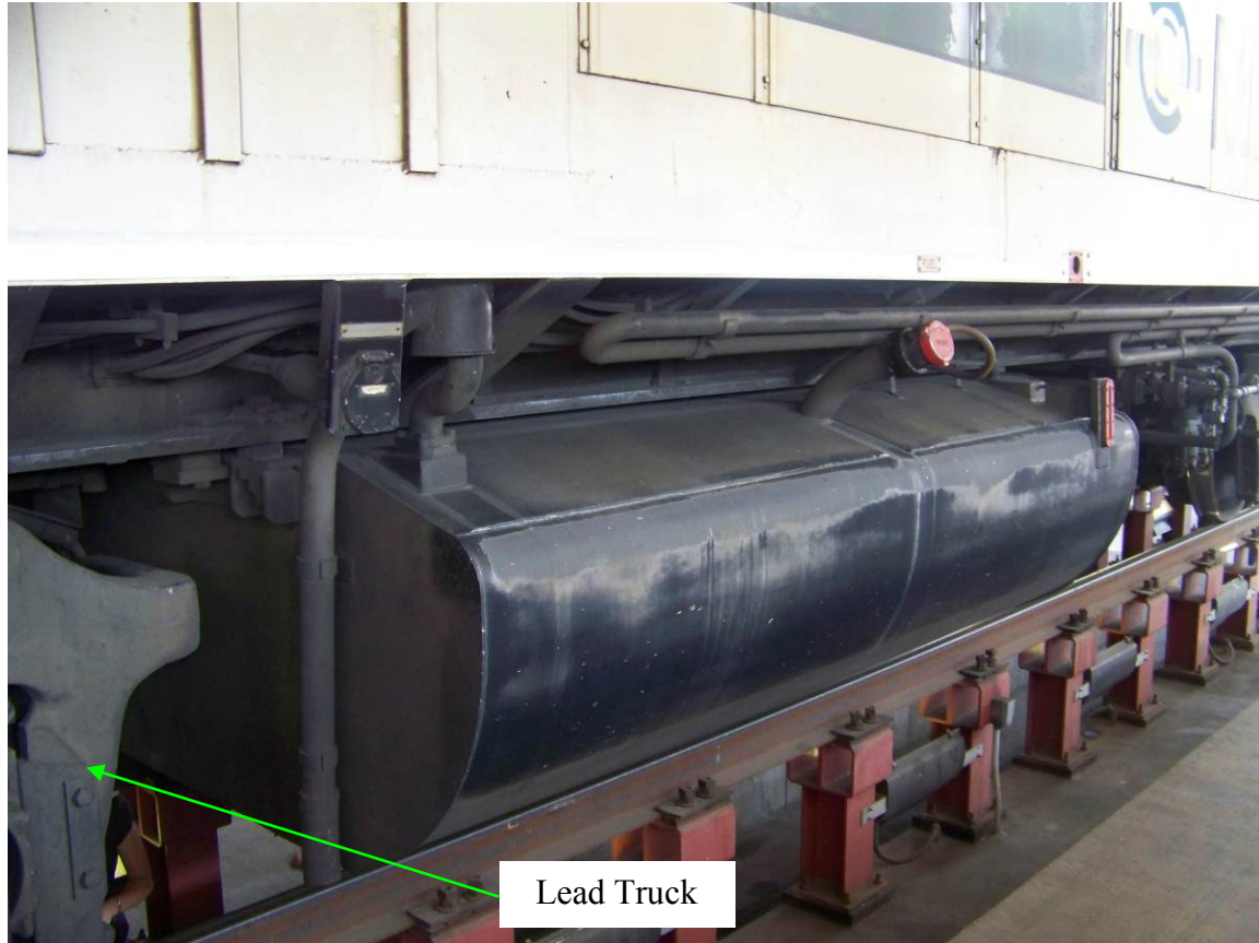
Figure A.3-1. Exemplar Passenger Locomotive Fuel Tank
