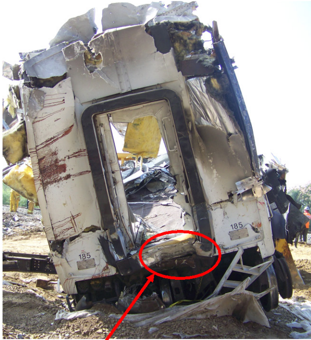
Indentation from Locomotive Bellmouth
