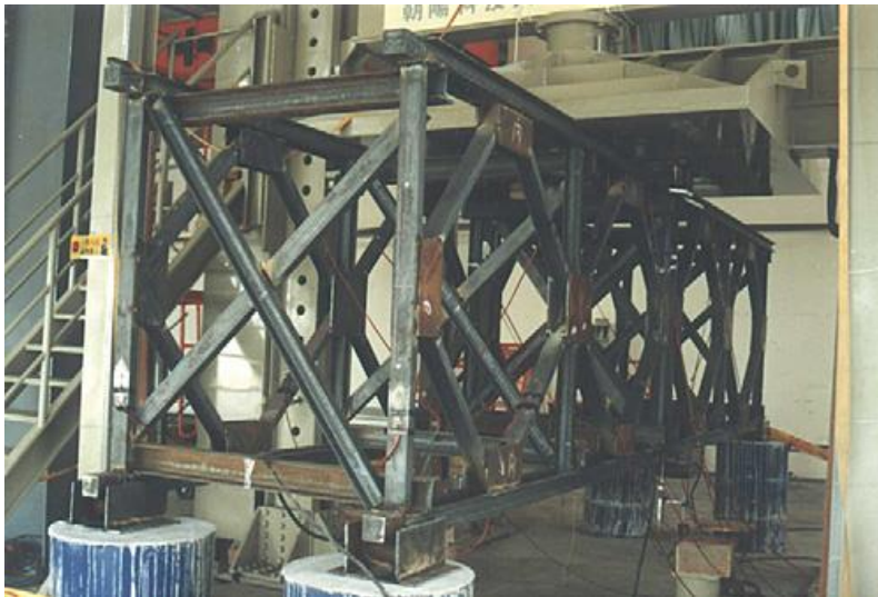
Full-Scale Bailey Bridge Model (King et al. 2013)
