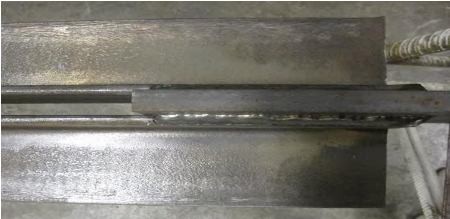
Double angle connection, Battistini et al. 2014
