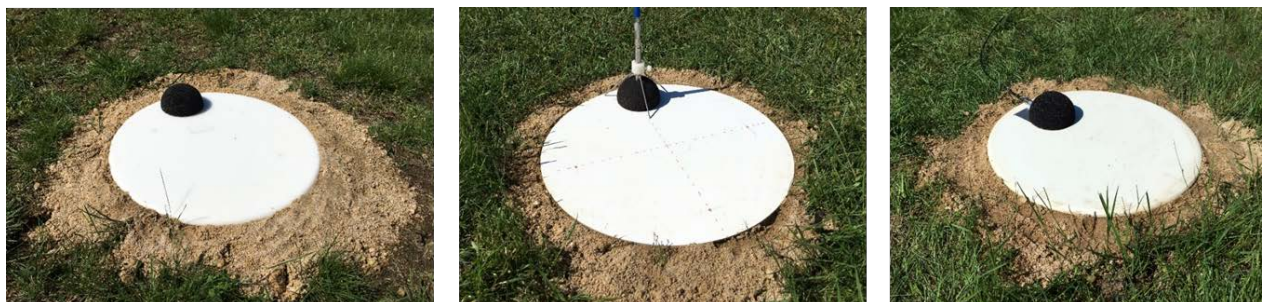
Fig. 4 - Ground plane and microphone configurations during an sUAS flight test
