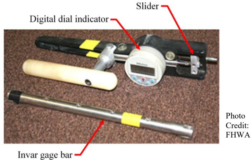
Figure 8. Photo. DEMEC Instrument and Gauge Bar.
