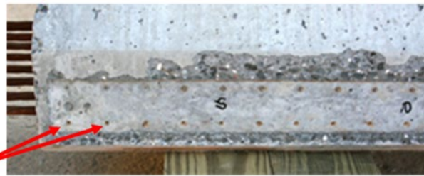
Figure 7. Illustration. Compound Figure Showing DEMEC Points on Girder End.
