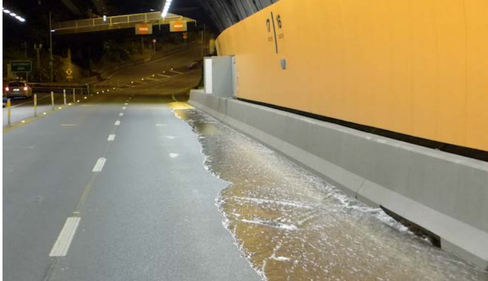
Figure 2-10: Water overflowing a drain in the Terrace Tunnel during an FFFS test.
