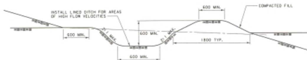
TYPICAL DRAINAGE SWALE
