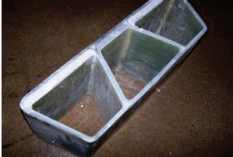
Figure 2. Photo. Basic configuration of a prototype of the hybrid deck.
