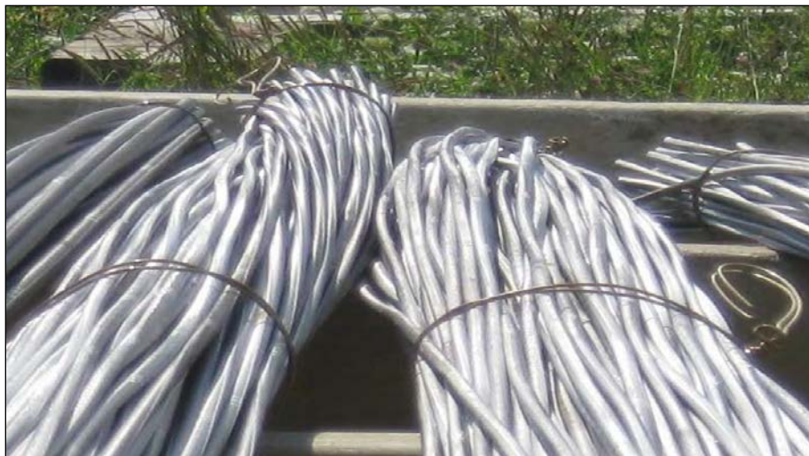
Figure 20. Condition of stainless steel rebar upon arrival.
