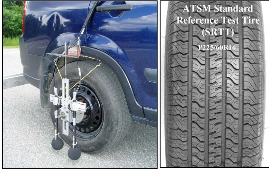
Figure 32. OBSI dual probe system and the SRTT.
