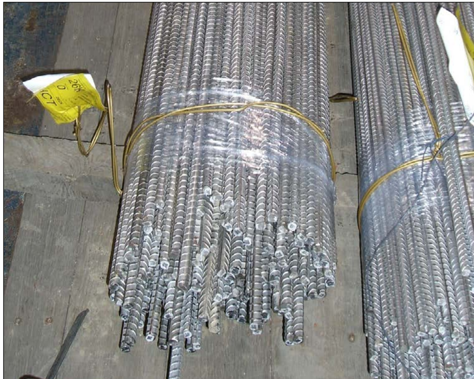
Figure 23. Stainless steel reinforcing bars prior to placement.
