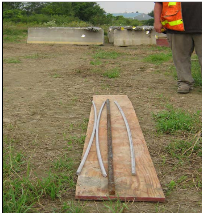
Figure 22. Curved condition of stainless steel rebar.
