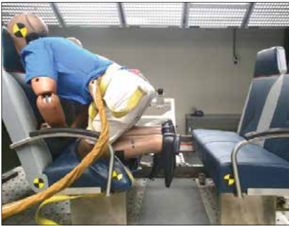
Photos show anthropomorphic test devices pre- and mid-test. Source: MGA
