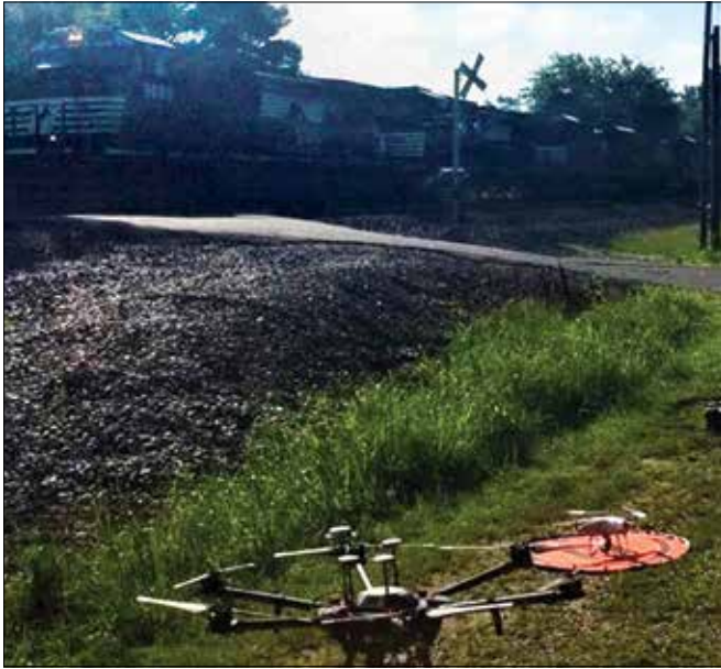
UAV equipped with LiDAR is ready to take off and survey an elevated grade crossing in Suffolk, VA. Source: U.S. DOT Volpe Center
