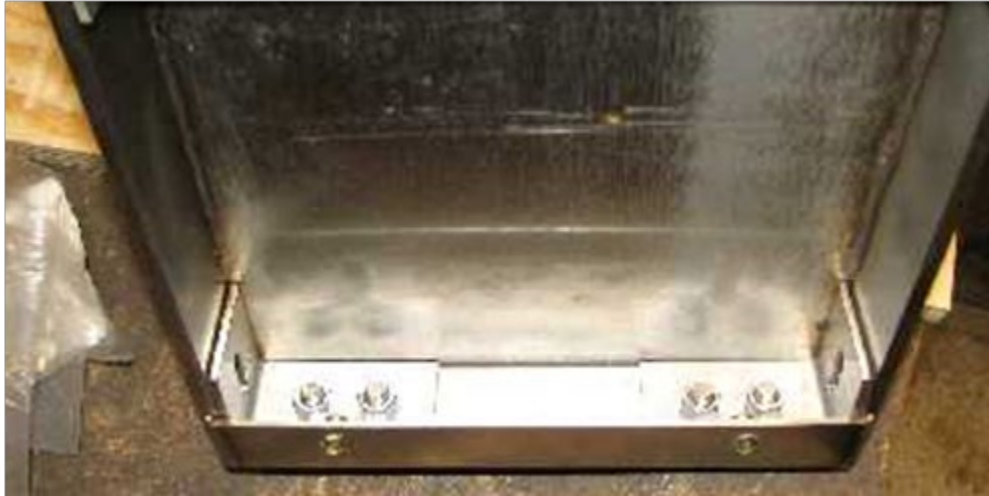
Figure 52. Assembled corner brackets in the revised pedestal
