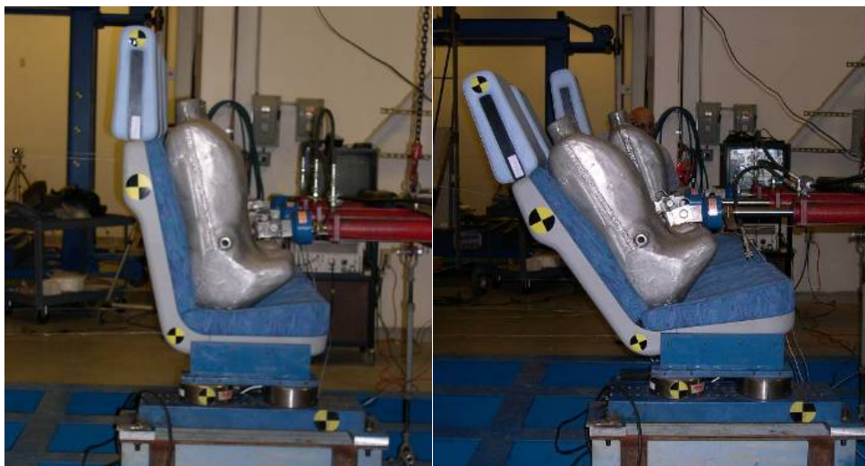
Figure 58. Pre- and post-test photographs of the RF body load test
