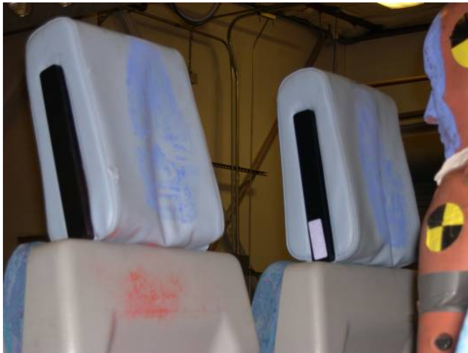
Figure 66. Impacted headrests following the FF dynamic sled test
