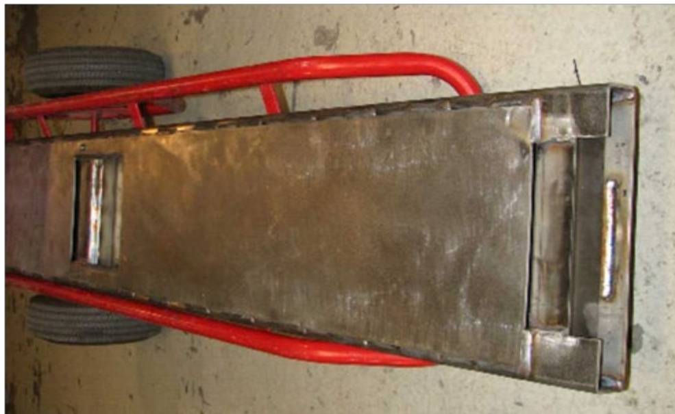
Figure 53. Seat channel with welded bottom cover plate
