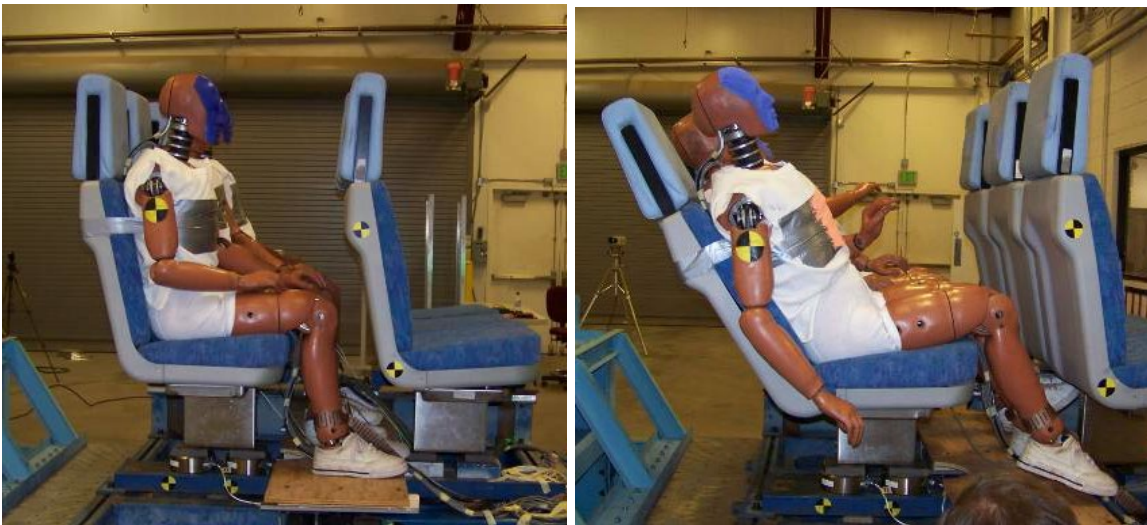
Figure 70. Pre- and post-test photographs of the RF 12g sled test
