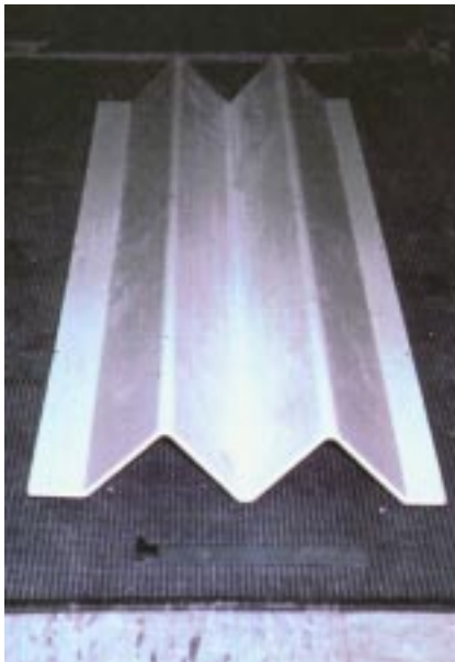
Figure 10. Commercially available pultruded FRP section of W-configuration, used for initial test (layup unknown).
