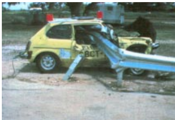
Figure 14. BCT speared on a 817.2-kg (1800-lb) car.
