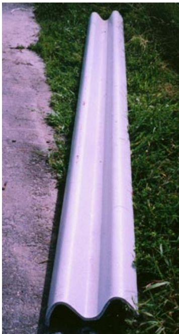
Figure 20. FRP W-beam as produced from the design.
