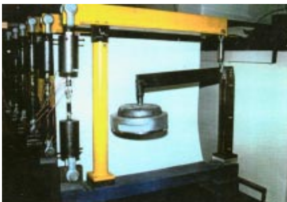
Figure 59. Creep test platform with six creep test fixtures.
