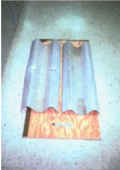
Figure 9. Tested (left) and untested (right) AASHTO W-beams. Note the local “yielding” as the energy absorption mechanism in these beams.
