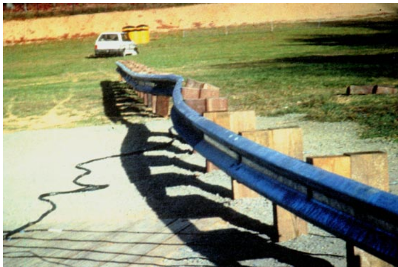
Figure B1. Crash testing of RPC posts and blockouts at the FHWA FOIL Laboratory.
