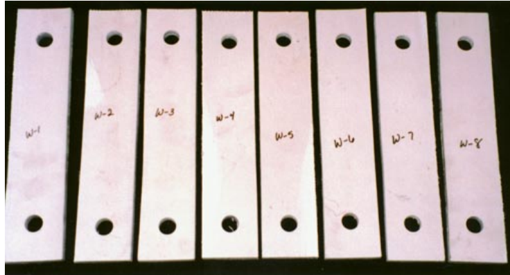
Figure 23. FRP W-beam test coupons for 19.05-mm (0.75-in.) bolt pull-out tests.
