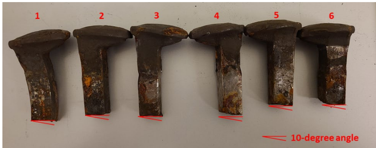
Figure 23. Orientation of cut spike failure plane
