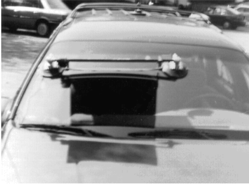
Figure 4. Windshield shutter installed on the Taurus test vehicle (Up or Open Position).
