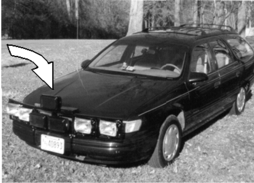
Figure 2. UVA headlight configuration on the Taurus test vehicle.
