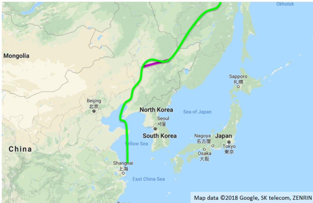
Figure 6-15: Flight 3 second lateral deviation with as-flown trajectory (green) and original planned trajectory (magenta)
