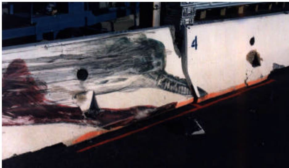
Figure 2-13 - Post Impact Scuff Marks Test 551
