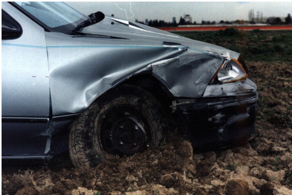
Figure 2-25 - Side Impact Damage
