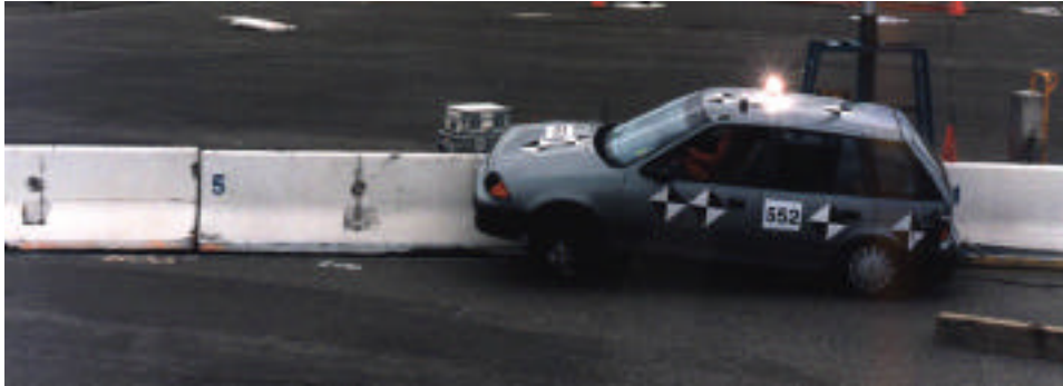
Figure 2-21 - Vehicle 552 Impacting Barrier
