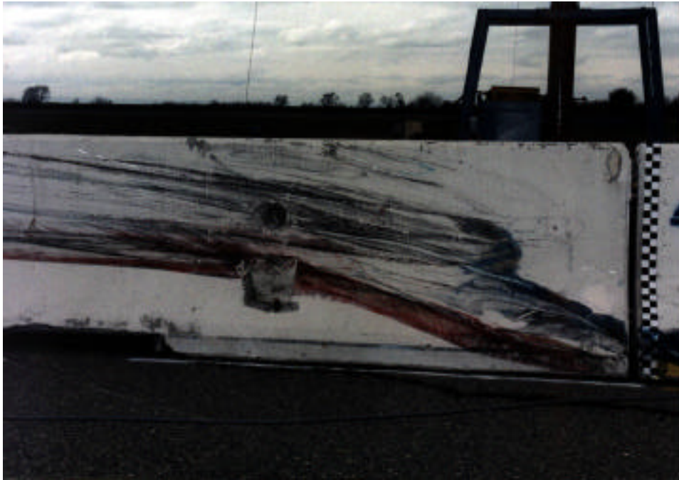
Figure 2-26 - Test 552 Barrier Scuffing
