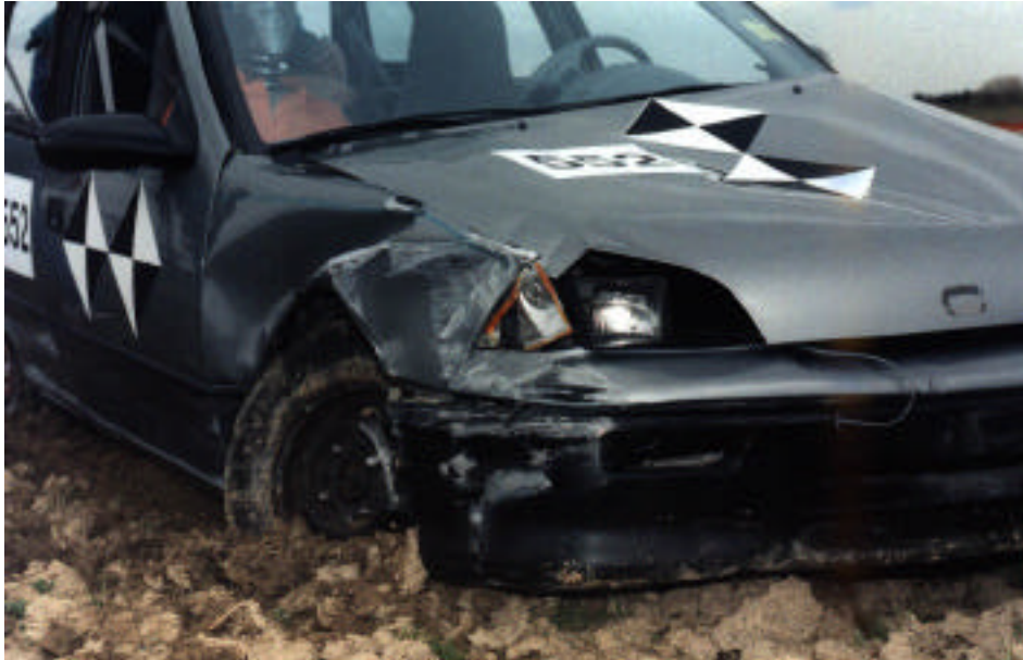
Figure 2-24 -Front View of Vehicle Impact Damage
