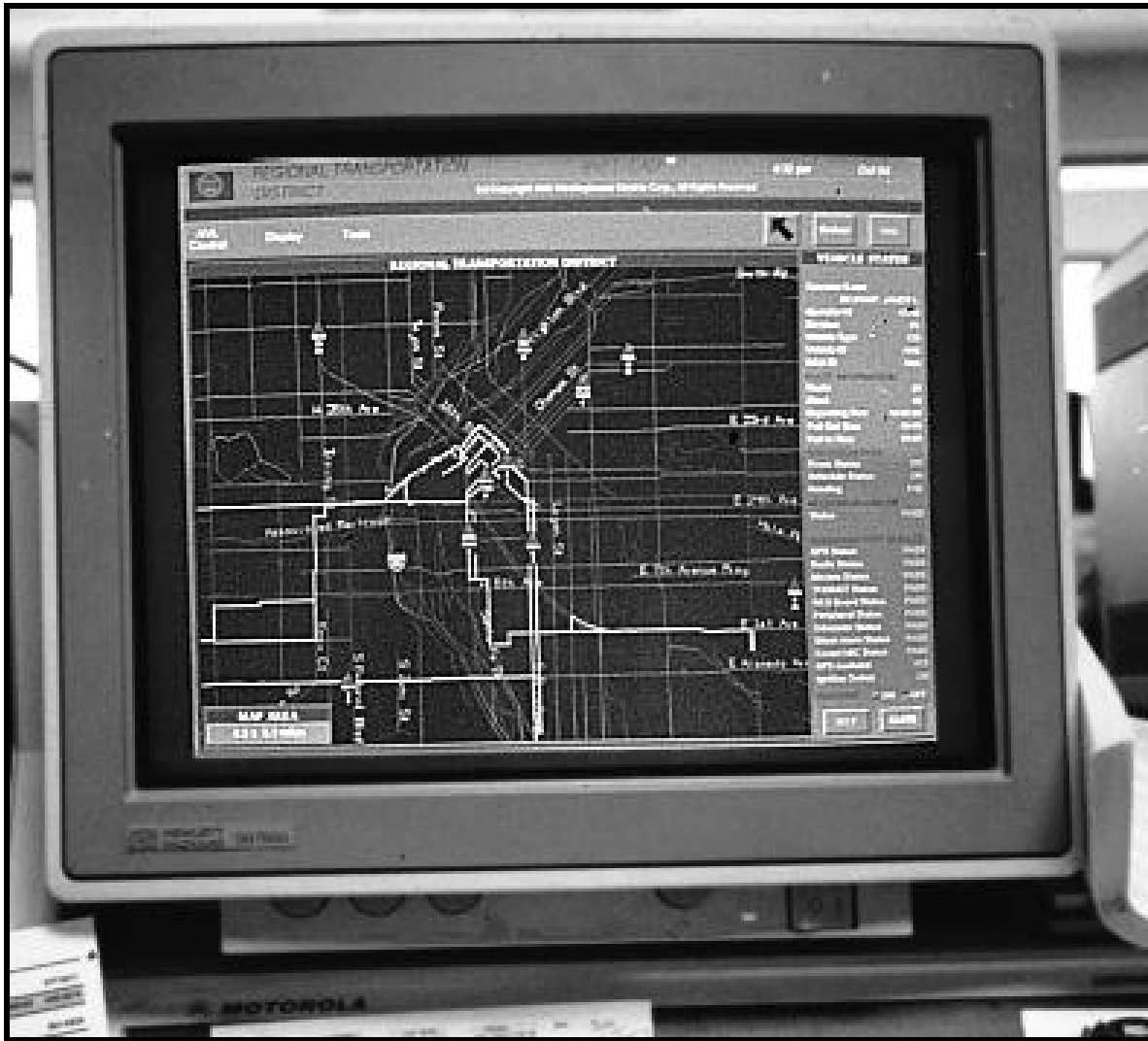
Figure 13. Automatic Vehicle Location Screen
