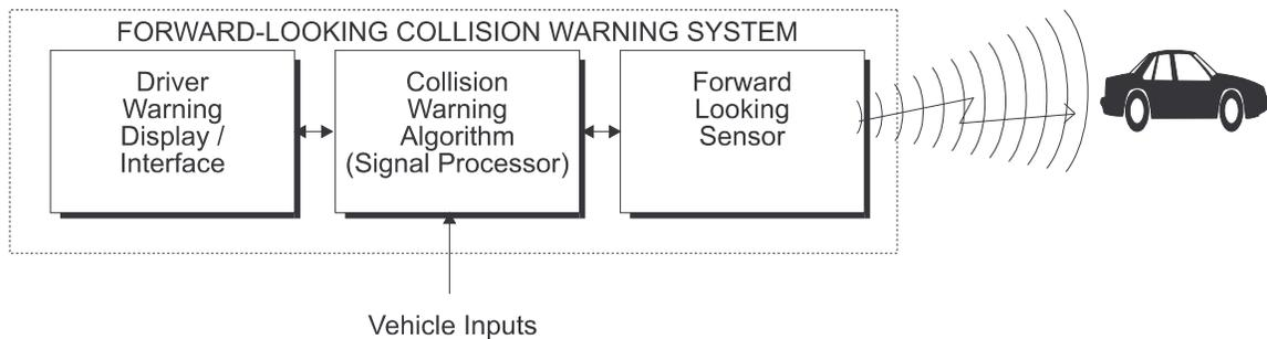
Figure 1 Forward-looking Collision Warning System Block Diagram
