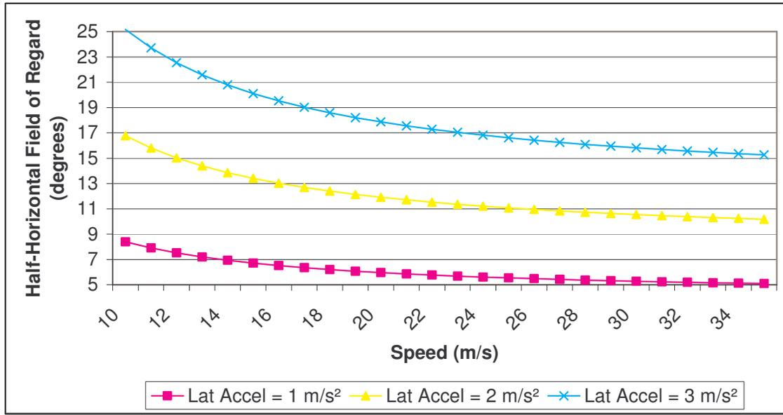
Figure 19 Half-Horizontal Field-of-regard versus Lateral Acceleration
