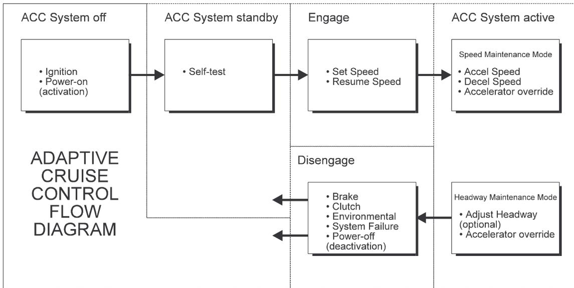
Figure 49 Adaptive Cruise Control Flow Diagram
