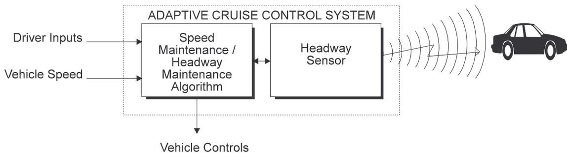
Figure 47 Adaptive Cruise Control System Block Diagram
