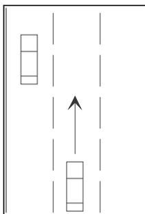
Figure 36 Adjacent Lane False Alarm Test Setup
