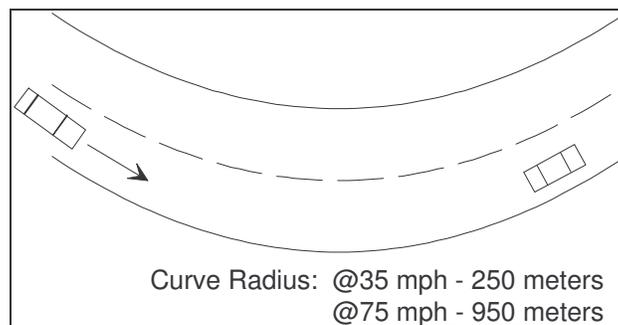
Figure 44 Tailgating Warnings on Curved Roads Test Setup
