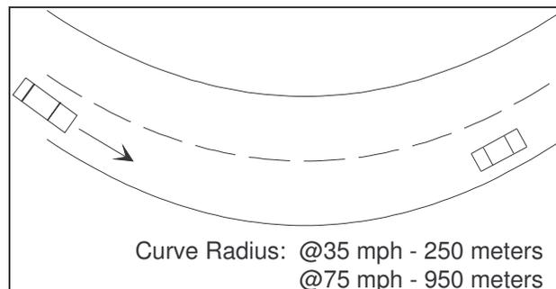
Figure 33 Curved Road Warning Distance Test Setup
