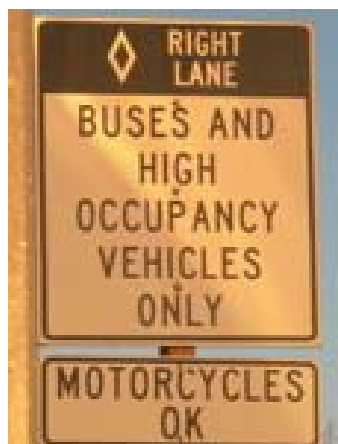
Figure 10-17: Metered HOV Lane Sign
