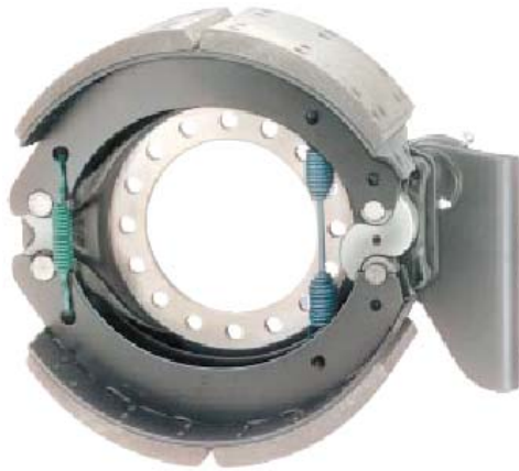
Figure 2.2-5. Typical S-cam Drum Brake (drum omitted for clarity) (ArvinMeritor photo)
